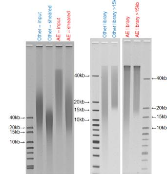
Pulsed-field gel electrophoresis demonstrated that gDNA from *E. coli* K12 strain MG1655 prepared by Amplicon Express (AE) was less fragmented than that from another commercial supplier (Other). Sheared AE gDNA also exhibited larger fragment sizes, as did SMRTbell™ libraries prepared from AE gDNA. No difference in library yield, either before or after size-selection, was seen (not shown).
